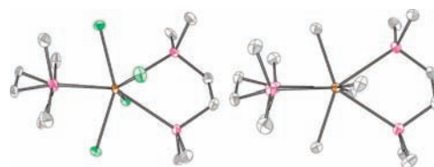
Figure 1. Molecular structures of the U(IV) phosphine complexes in compounds 1 (left) and 2 (right), rendered with 40% ellipsoids. Brown, purple, green, and gray ellipsoids represent U, P, Cl, and C atoms, respectively. Hydrogen atoms are omitted for clarity.
